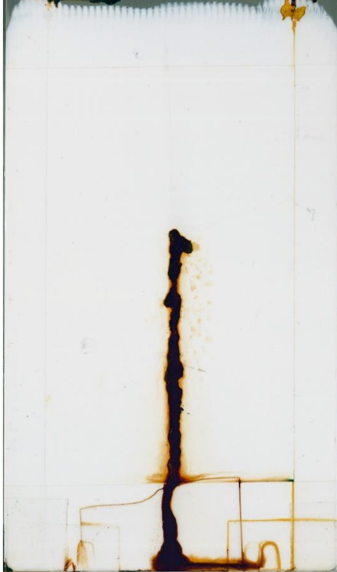
1440h NSST, Gardobond OC panel, approx. 110 \mu m DFT
